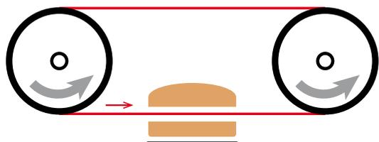
*Slicers designed to slice sponge cake are equipped with continuous band blades for sharp, smooth and clean cut. In addition to the standard versions, others can be available, on order, in which the slicer can be equipped with one or more cutting heads in line for the multiple cut of the product in layers as required by client needs.*
